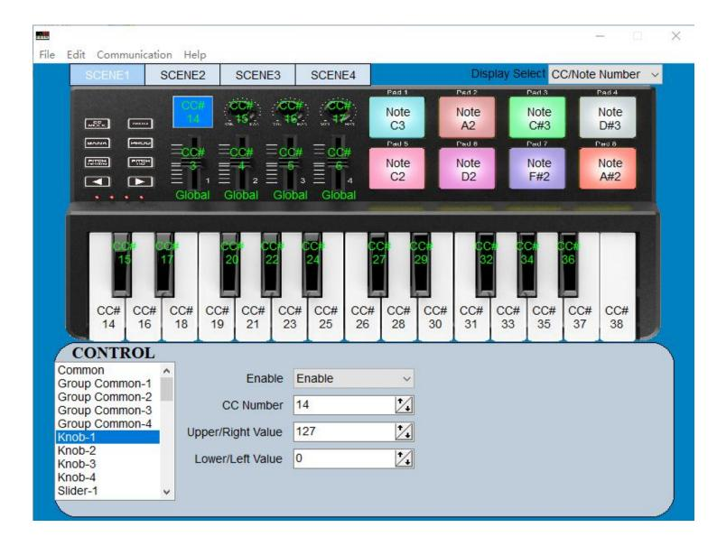
Operating a knob will transmit a control change message. You can enable/disable each knob, specify its control change number, and specify the values transmitted when the knob is turned fully left or fully right..
