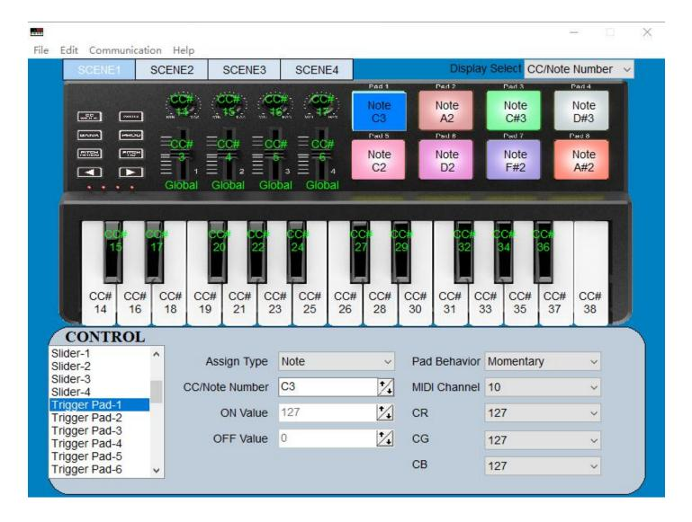
Depending on the assign type, the trigger pads can transmit note messages or control change messages. For each trigger pad, you can individually specify the assigned message, the MIDI transmit channel, the behavior of the trigger pad, the note number, the control change number, the values transmitted when the pad turns on or off.
