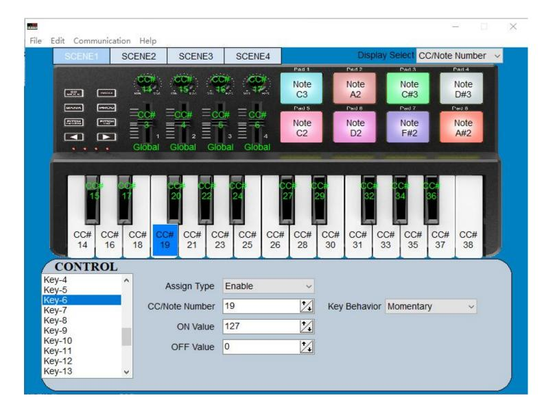
The twenty-five keys of the keyboard will function as independent buttons to transmit control change messages. You can specify which MIDI channel the control change message is transmitted on, whether or not each key is enabled, the key type, the control change number, as well as the On and Off value.
